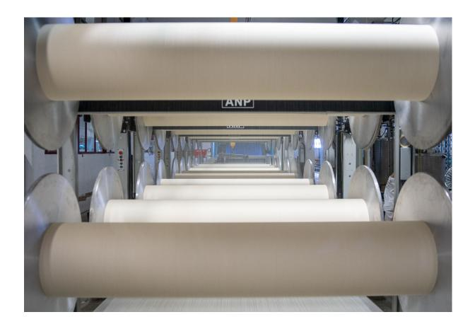
When unwinding the heavy warp beams with a diameter of up to 1400 mm- often with few threads- it is important to keep the thread tension constant during stop, acceleration or production speed.
