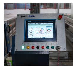
The system is operated via several redundantly working HMIs, via which all machine functions can be accessed, helping the operator to supervise and execute all operations in the safest condition, keeping the whole process under control. This also has the advantage that if one HMI fails, the system can continue to be used at any time via the other devices, thus avoiding machine stops.
