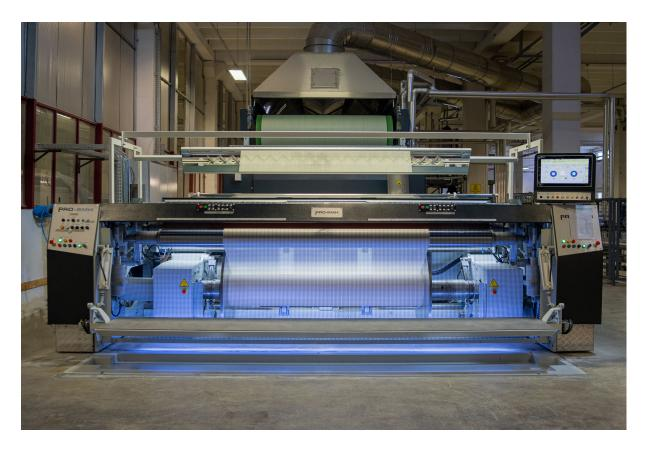
One of the core elements of every sizing system is the headstock. An absolutely even and controlled structure of the warp with exact maintenance of the desired tension is a key to effective and trouble-free work in the weaving department.
