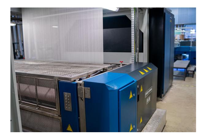
SMH  $\dot{v}$  - Sizing® sizing machines with intelligent computer system produce weaving beams
