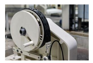
The **AP®** unwinder is used to feed warp beams from sectional warping machines to the sizing machine. Of course, while maintaining perfect tension regulation from the first to the last meter.
