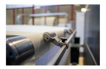
The speed of the system is controlled by maintaining a constant, adjustable residual moisture content in the yarn. This unit is integrated and operated completely via the machine control of our system.
