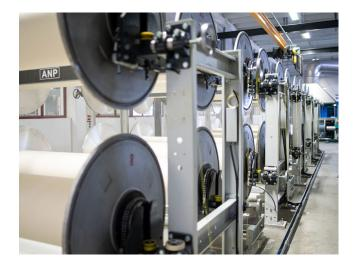
And this, of course, from the first to the last meter of yarn on the respective warp beam. With the types **ANP®**, **ANV®** and **AM®**, PRO-SMH offers beam creels that are optimally tailored to the needs of the user and fully meet the requirements described before.
