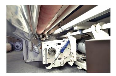
Depending on the desired diameter of the weaving beam, the beaming machines **PT-10**® (ø 1,000 mm), **PT-11**® (ø 1,110 mm) and **PT-12**® (ø 1,250 mm) provide the operator with the ideal and reliable tool. The working range can be selected in the range from 800 to 4,600 mm.
