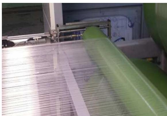
Entry and exit rollers, with pneumatic activation, allow accurate adjustment of the motors as well as a damping system to keep the yarns guided without any stress.
