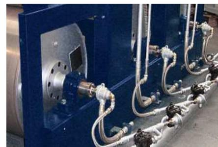
Size is kept at the best temperature for yarn's impregnation and reaction to the pre drying units.
