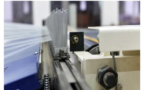
Constant warp laying on the beam is a key factor, particularly with anelastic yarns. Each individual filament passes through the machine with a clearance of 1 to 1.5 mm from the adjacent filament.
