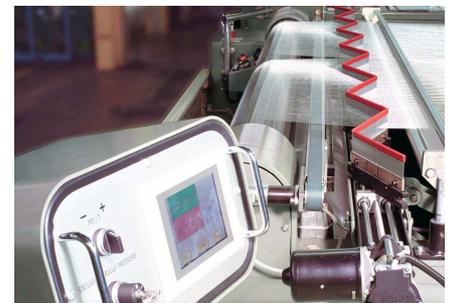
Constant warp laying on the beam is a key factor, particularly with anelastic yarns. Each individual filament passes through the machine with a clearance of 1 to 1.5 mm from the adjacent filament.
