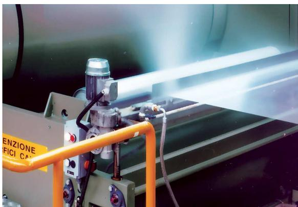
Entry and exit rollers, with with load-cell, allow accurate adjustment of the motors as well as a measuring system to keep the yarns guided without any stress.
