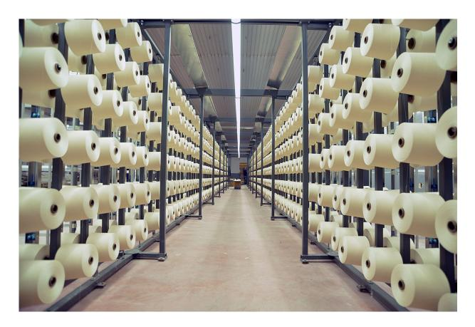
The **PRO-H-CREEL**® portfolio of PRO-SMH is based on a modular design and offers different models, swivel creels for large and heavy packages, truck-trolley creels for highest productivity and magazine creels with thread transfer for continuous production. Both outside and inside threading is available in all types and layouts.
