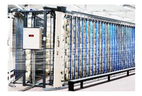
Our modular construction guarantees an easy erection of the creel and allows creel enlargements and displacements to other departments. To accommodate the limited space, we can also manufacture creels on two decks, equipped with access staircases and elevators. Movable creels are also available.
