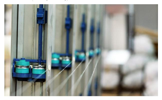
The **PRO-TT-DISC**® achieves perfect warps by ensuring absolutely constant thread tenisons regardless of the package diameter or the speed. The tension is achieved by applying pressure on the upper disc of the second set of discs. The first set of braking discs ensures stable movement of yarns and makes it possible to apply proper tensions afterwards.
