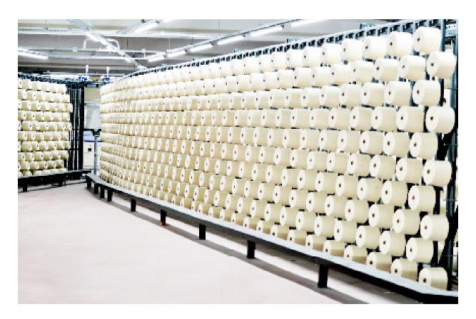
The **PRO-V-CREEL**® from PRO-SMH is highly suitable for processing all cotton, spun rayon and blended staple fiber yarns up to a speed of 1200 m/min.
