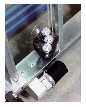
Caps rotation: The rotational movement, centralized for each side of the warping creel, is transmitted to the caps by means of particular gearing. The controlled rotation of the caps ensures their perfect cleaning and exceptional durability.
