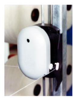
Caps rotation: The rotary movement, centralized for each side of the warping creel, is transmitted to the caps by means of a through-shaft and by gears and pulley transmission. The controlled rotation of the caps ensures their perfect cleaning and exceptional durability.
