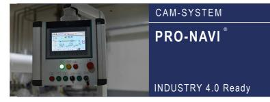
LAN communication (Ethernet) is possible from the machine, so such as operation check, production record, and monitoring can be easily made by managers in the office. This Navigation system is Industry 4.0 ready and makes your investment even more profitable.
