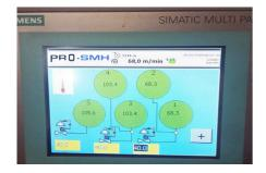
Size is kept at the best temperature for yarn's impregnation and reaction to the pre drying units.
